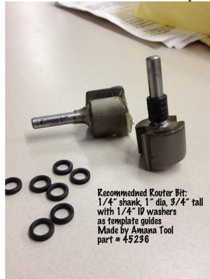
8. Use Router with suggested bit to rout cavity along front, back and sides of Pocket Rout template. I use Two templates to set the depth of the router. 0.44". When locked at that depth, and using the pocket rout template on the guitar, it leaves the original shape of your cavity as it was, and starts the rout 0.22" below the back of the guitar.
