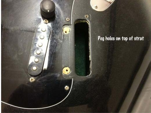
2. Most strats will need a touch on the top rout in order for the Trem King unit to center properly. The diagram below shows placement of the top rout template and pocket rout. We recommend Low Stick masking tape to cover areas to be marked.
